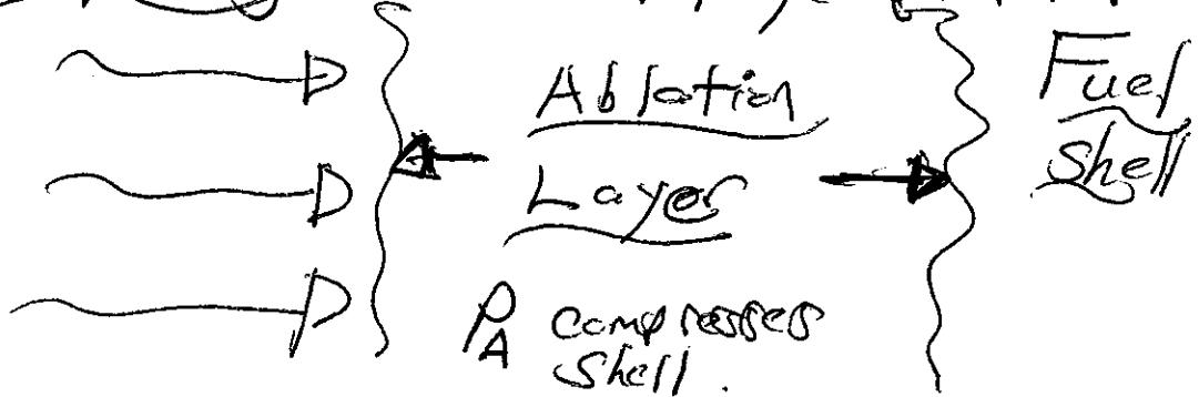
Note: "implosion" is just conservation of momentum between expanding ablator layer and inner shell
