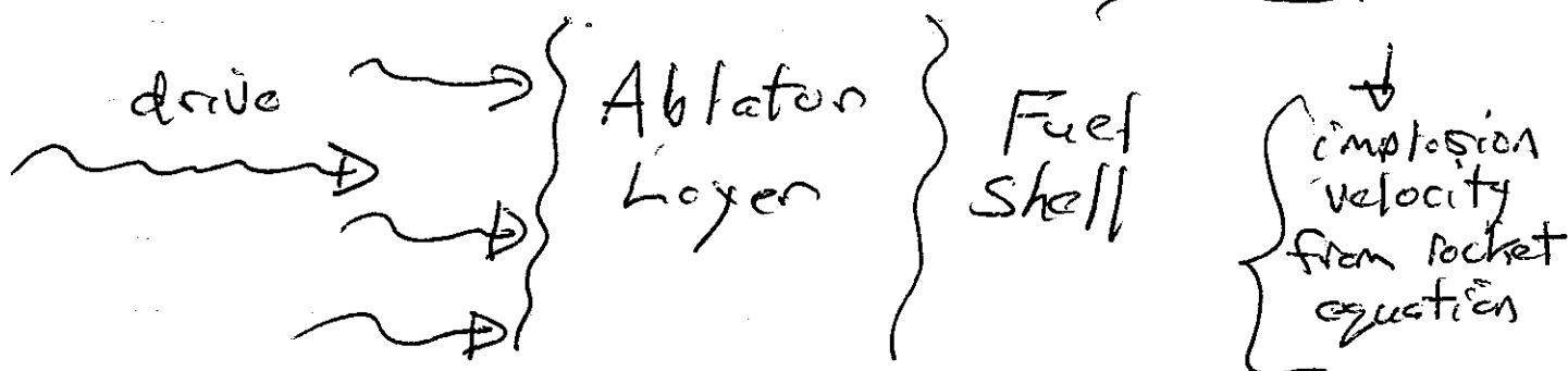
ablator layer heats and expands thus compressing inner fuel layer (via PV work)
